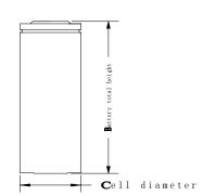
Cell diameter  $18.2 \pm 0.2 \text{ mm}$
