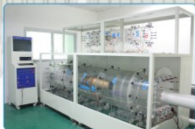
风洞实验室 Windtunnellaboratory One: 0~100CFM, 0~100mmAq Two: 50~2000CFM, 0~250mmAq
