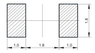
Note: It is recommended that the metal stencil used for solder paste printing has a thickness of 0.1mm (4mils) or 0.12mm (5mils).
