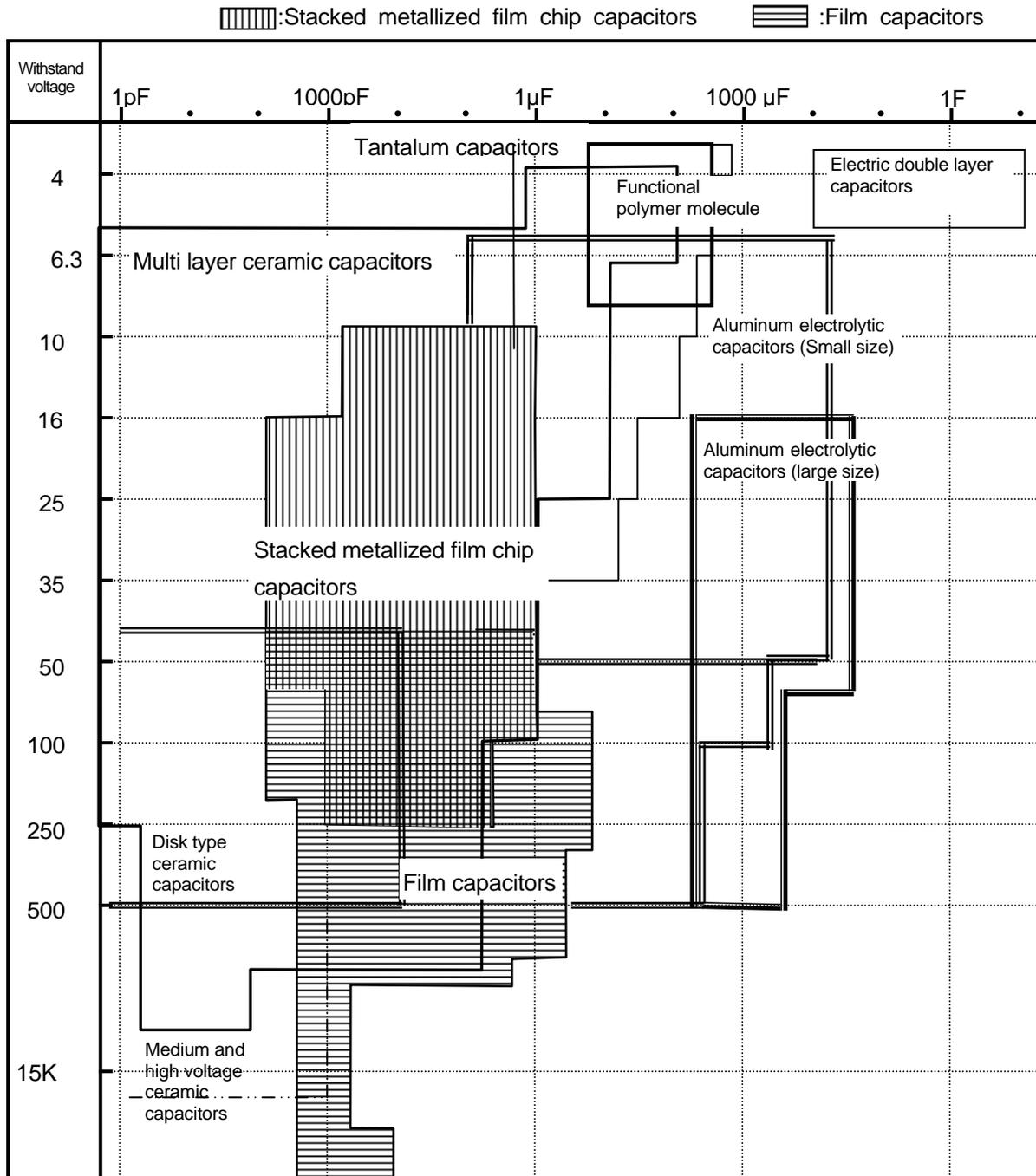
Note) This chart shows just a typical example. Capacitors with capacitances and rated voltages other than this chart are also available.
