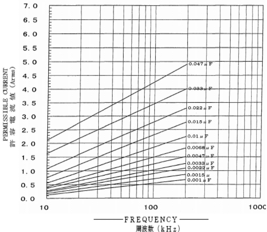
Derate the permissible current value if the wall temperature of capacitor become over 85 degree C as the following figure shows.
