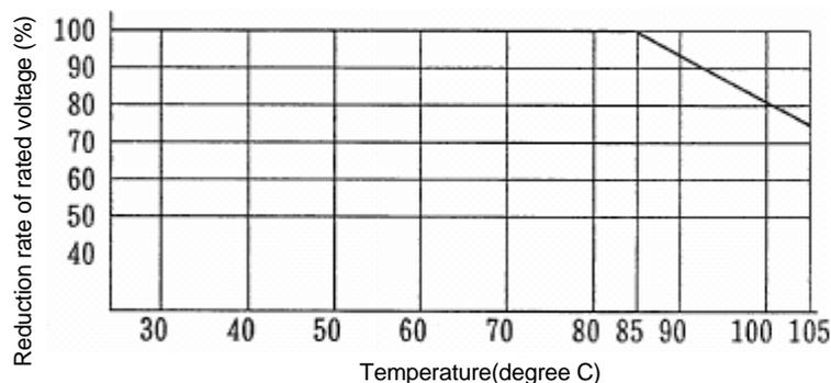
Fig.16 Rated voltage derating against temperature of ECQE(F)
