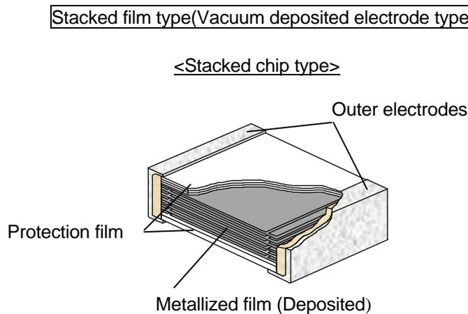
**Fig.5. Structures of various types of film capacitors**
