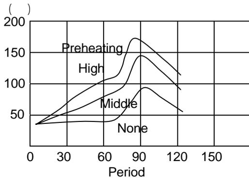
**Fig.19. Element temperature change due to preheating**
