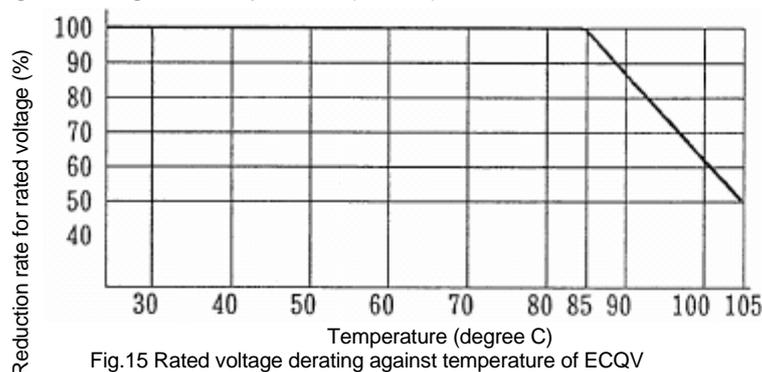
Fig.15 Rated voltage derating against temperature of ECQV
