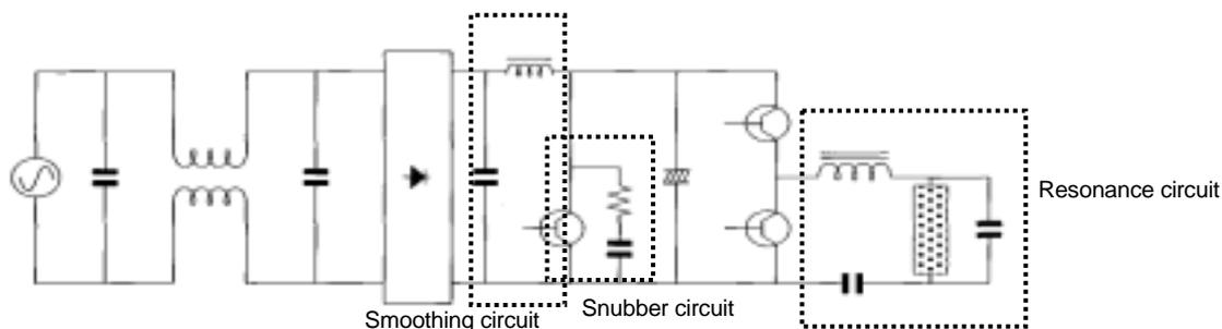
Switching element brings pulse generation in snubber circuit to generate high frequency. Film capacitors remove noise in switching.
