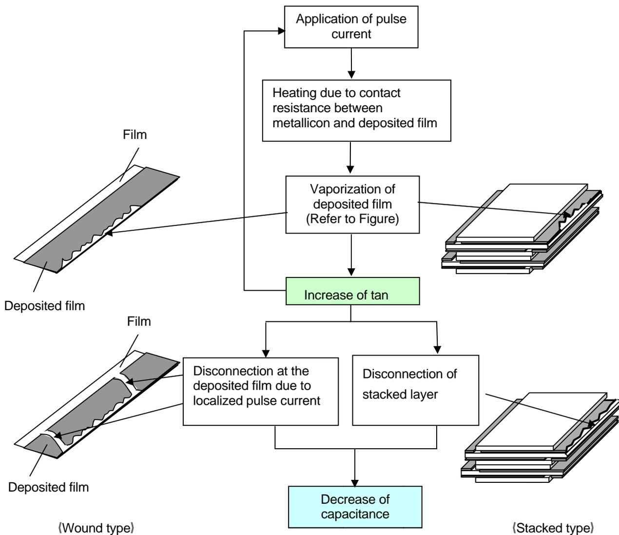
**Fig.9. Failure mechanism by pulse current**
