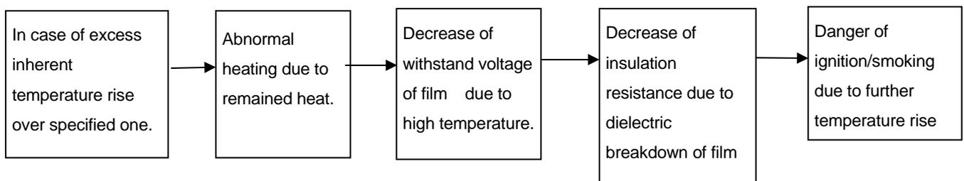
Fig.11 Breakdown mechanism by continuous current
