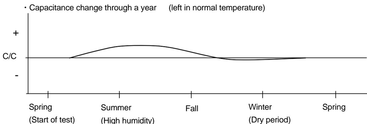
Fig.18 Capacitance change through a year (left in normal temperature)
