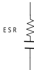
(Equivalent series resistance: Series resistance by film characteristics, Lead wire resistance, Contact resistance of metalicon, Electrode resistance)
