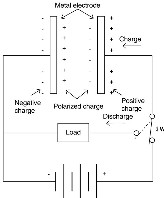
Fig.2. Principle of capacitors
