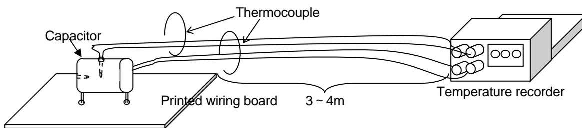
**Fig.22. Test method of element temperature profile in mounting**
