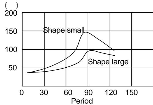
**Fig.20. Element temperature change according to element size**
