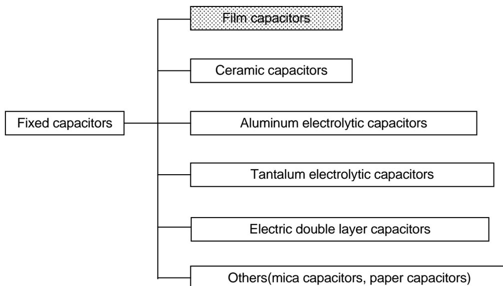
Fig.3. Typical classification of fixed capacitors according to type of dielectric materials
