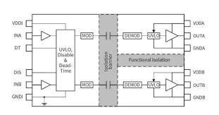
Block diagram of NSI6602 Isolated driver system
