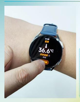
Xiaomi released its S2 smart watch in December 2022. The watch is equipped with two NOVOSENSE temperature sensors: NST112C-CWLR and NST112D-CWLR.
