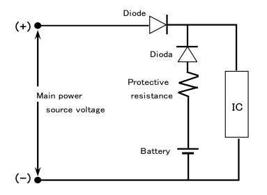
Back-current Prevention Diode and Protection Resistor Used
