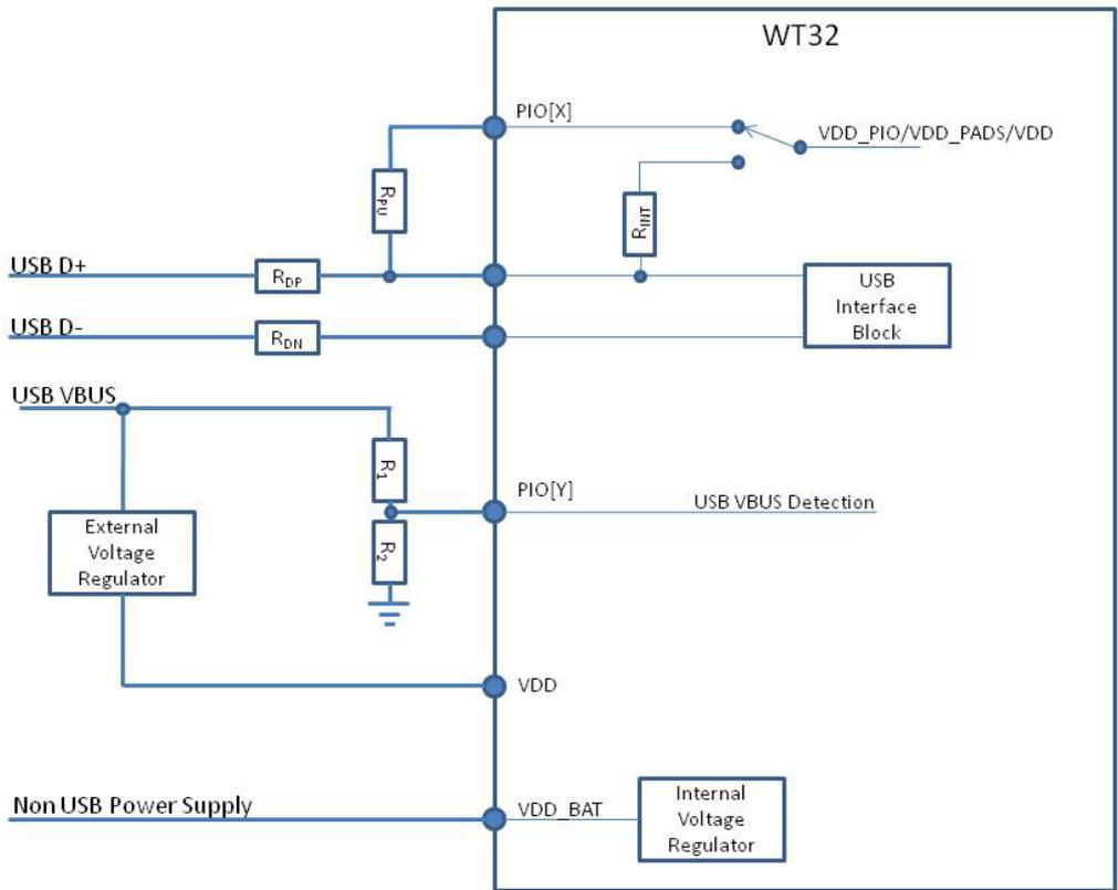
**Figure 5: Self-powered WT32 device**
